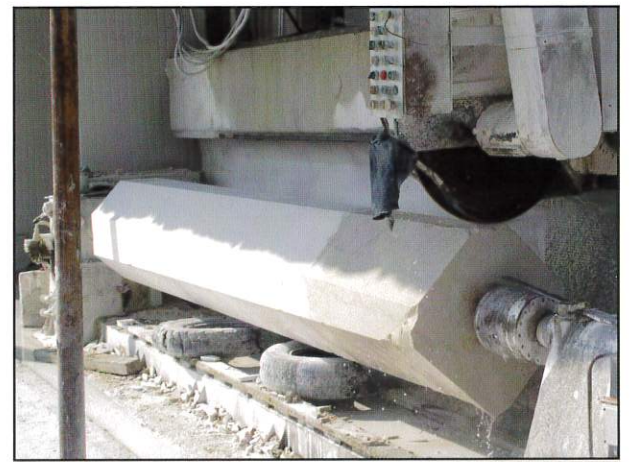
Each column was turned on a computerized lathe to achieve a cylindrical shape.
