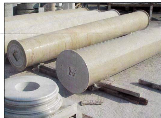
The nearly-finished products. When positioned on their bases in Our Lady of the Most Holy Trinity Chapel, the columns will stand 15 1/2' high.
